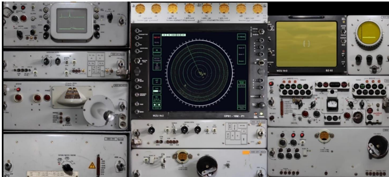
Figure 7: SA-8 operator station built in DSC controlling MACE entity SGE devices and receiving visuals from ARMOR
