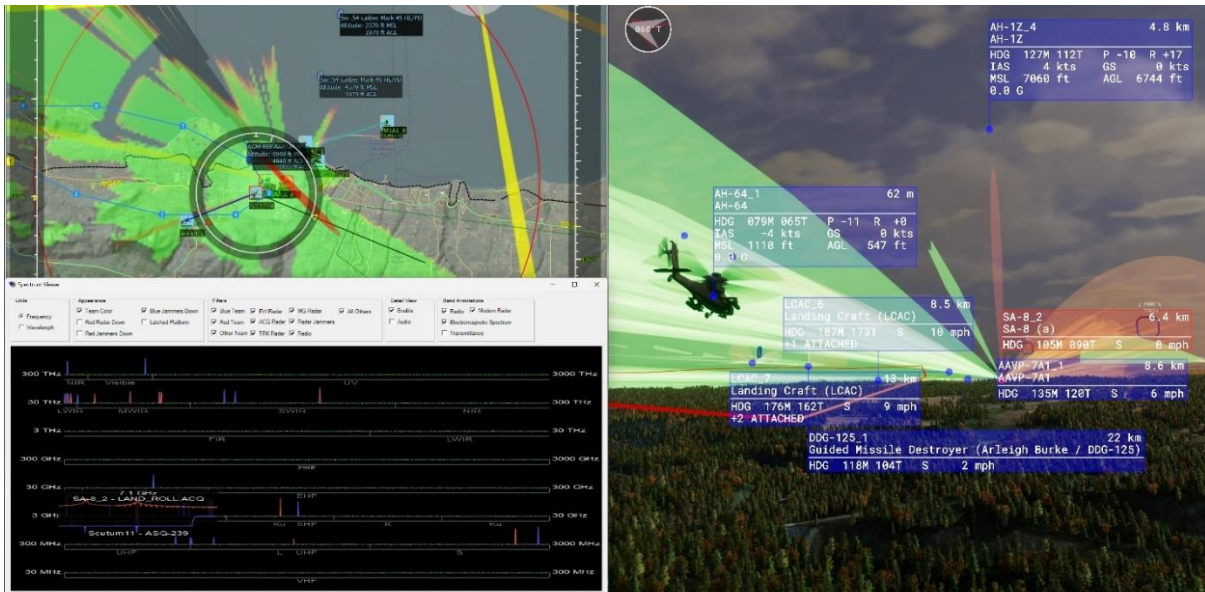
Figure 28: MACE and ARMOR visualizations showing beam shape, jamming corridors radar propagation; and spectrum analyzer
