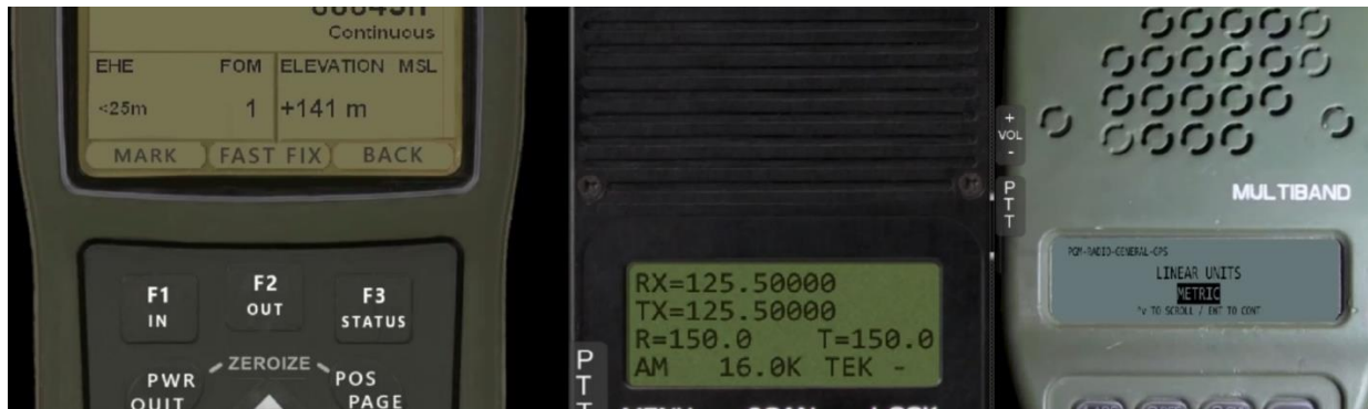
Figure 18: BSI Emulated Advanced GPS Receiver (B-EAGR), PRC-148 and PRC-152 Radios
