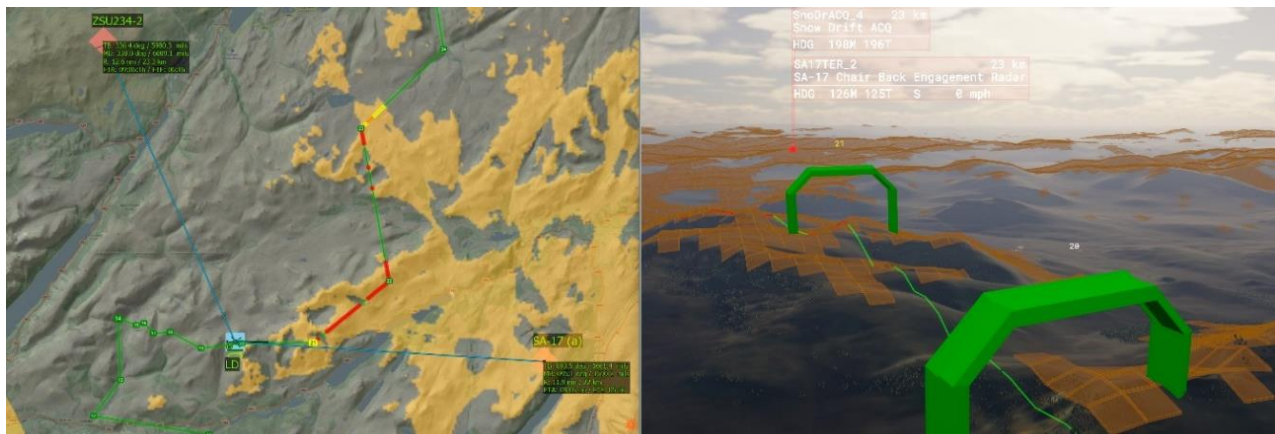
Figure 12: MACE (2D) and ARMOR (3D) route evaluation and Radar line of sight plots
