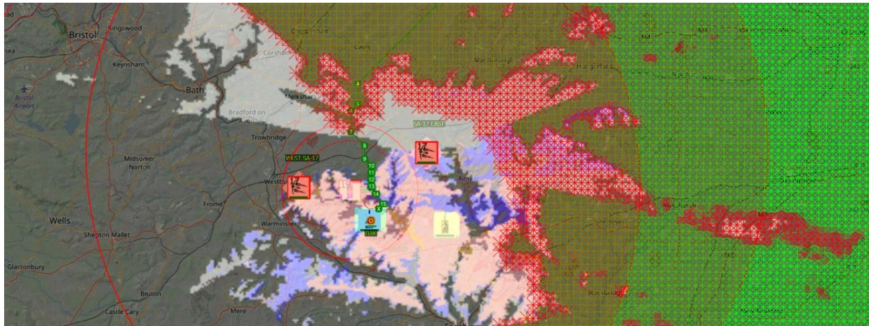
Figure 13: MACE Assisted Route Creation (MARC) in progress vs multiple threats to find optimum route
