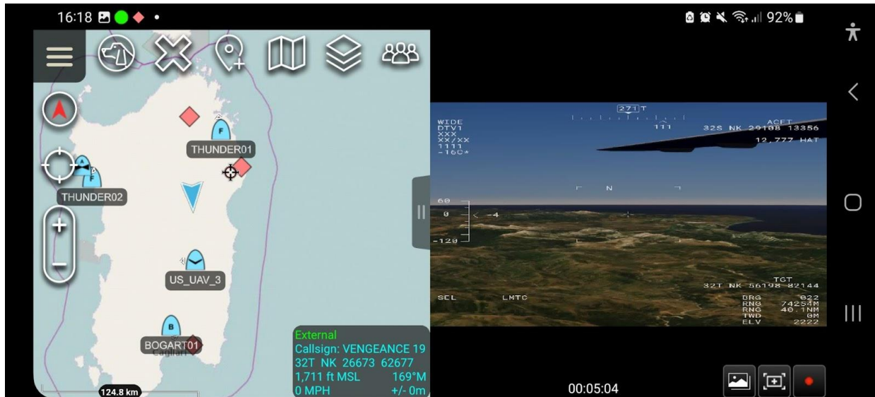
Figure 27: ATAK displaying MACE generated entities passed over COT protocol & ARMOR synthetic streaming ISTAR VDL
