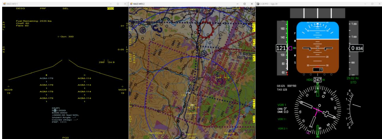
Figure 32: MACE Plugins used to create interactive tactical displays and primary flight instruments
